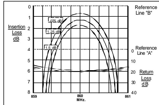
Figure 5 **Band pass cavity responses**
