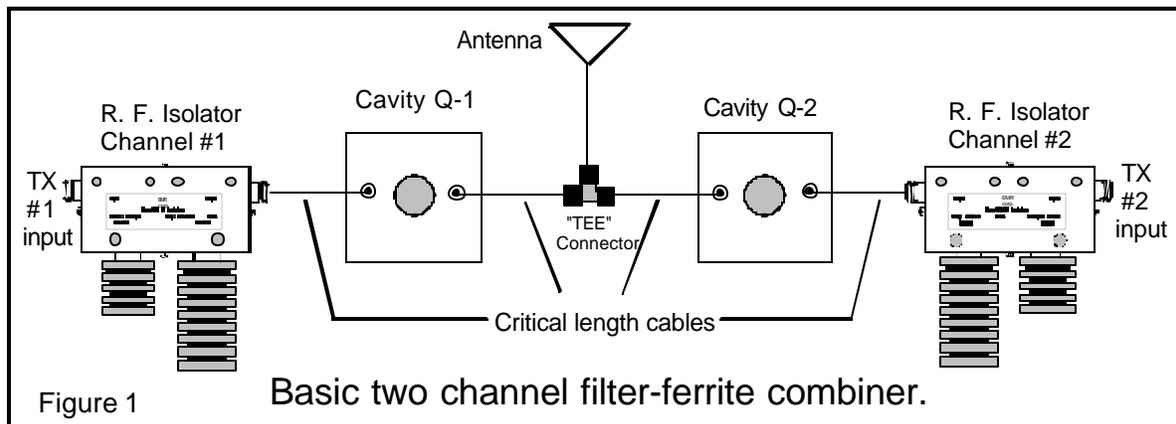
The design of this form of combiner is most often referred to as *Filter – Ferrite* since the major components are cavity filters and ferrite based isolators along with selected cables, connectors and hardware. First, we will review the nature of filter-ferrite combiners as an overview, then show how the various elements of this type of combiner contribute to the overall assembly.
