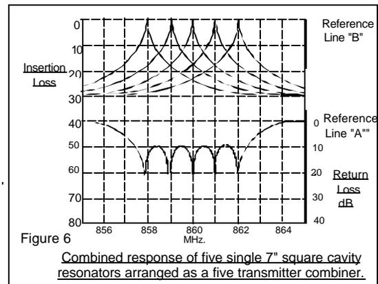
Figure 6 **Combined response of five single 7" square cavity**
