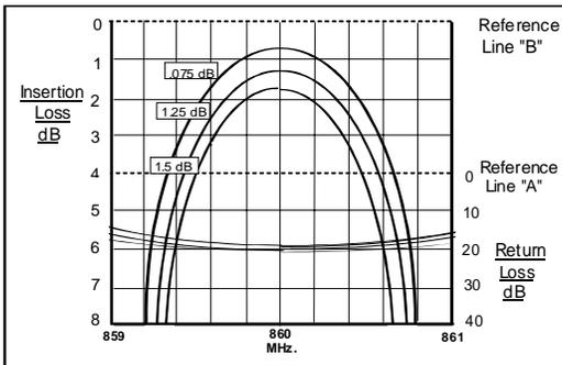
Figure 5 Band pass cavity responses
