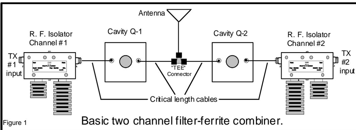
Figure 1 shows a basic two channel filter-ferrite combiner. A dual R. F. isolator feeds a band pass cavity in each branch. The outputs of the cavities are tied together with a "tee" connector for combining to a common antenna.
