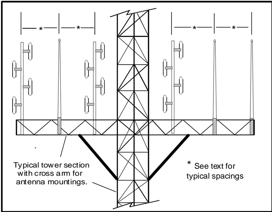
Figure 10 Horizontally Mounted Transmitting Antennas
