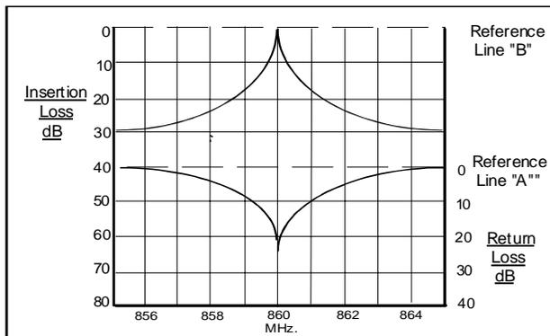
Figure 2 Response of single 7" square cavity
