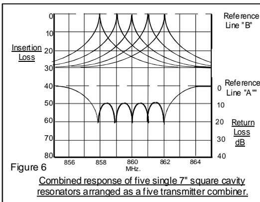
Figure 6 Combined response of five single 7" square cavity
