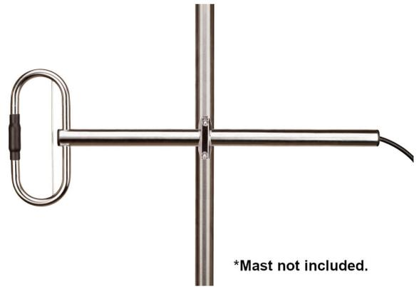
The EMR450DP single bay dipole is a rugged, all electropolished stainless steel, folded broadband dipole for use in the 360-520 MHz band. It is all stainless steel construction, suited to harsh environments. This antenna can be mounted in three configurations to allow for different shaped radiation patterns in the H plane, including 1/4, 1/2 and Full Wave length spacing from the vertical mounting pole.
