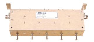
EMR Corp RF Preselectors vary from single or dual cavity resonator combinations, to mult-stage inductive, aperature coupled, or combline filters. Special preselector assemblies may include one or more of these devices in combination, multiple pass and stop band characteristics, and special notch elements according to the complexity of site requrements. EMR preselectors are designed to optimize loss, selectivity, and costs; with respect to the particular site requirements and frequencies.
