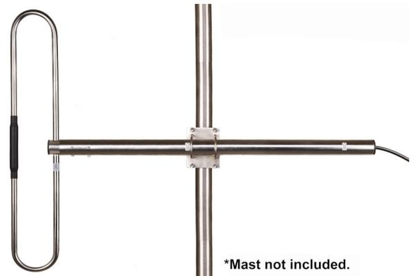
The EMR150DP antenna is a 2.5dBd gain, all electropolished stainless steel, folded dipole antenna for use in the High Band VHF Commercial Radio band. Its wide bandwidth is ideal in duplexing and multicoupling. Its robust construction ensures excellent longevity and performance. The all electropolished stainless steel construction is ideally suited for weather corrosion resistance.
